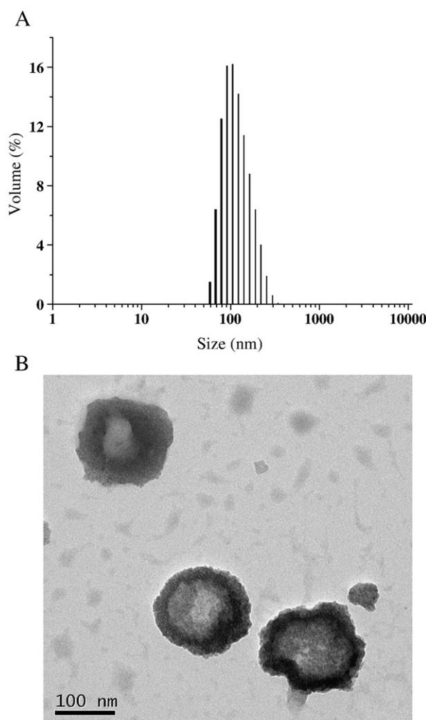
**Fig. 1.** Size distribution profiles for pH-sensitive degradable polymersomes (1 wt.% staining agent) determined by DLS (A) and TEM (B).
