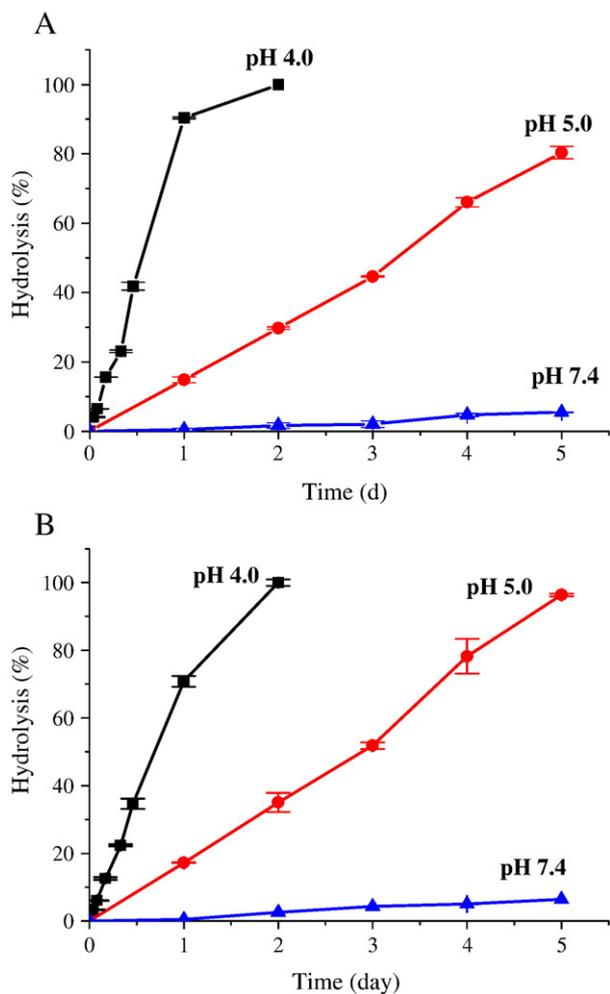
Fig. 3. pH-Dependent hydrolysis of acetals in the polymersomes (A) and micelles (B).
